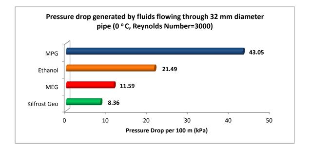
As the data shows, fluid flow with a Reynolds number of 3000 in a pipe of diameter 32 mm at 0  $^{\circ}$  C leads to the development of a pressure drop with all thermal fluids. However, the type of thermal fluid used determines the extent of the pressure drop. The data shows that Kilfrost GEO leads to the lowest pressure drops in the system. In consequence, Kilfrost GEO is hydraulically superior to MEG, MPG and Ethanol based thermal fluids.
