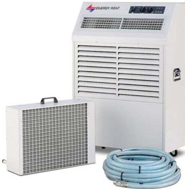
This compact unit consists of an indoor unit and an outdoor unit, which are connected by glycol-filled hoses quick connections. A pump that ensures circulation is installed. The indoor unit has high and low pressure alarms as well as an automatic defrost system. The condenser heat is conducted through them glycol-filled hoses to the outdoor unit. KM 7 Cool is extremely flexible and is perfect for cooling server rooms, for use at events and in shops.
